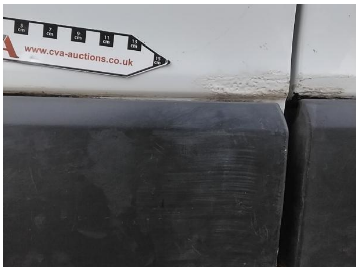
8: Door nsf Scratched UpTo 25mm Thru Paint
