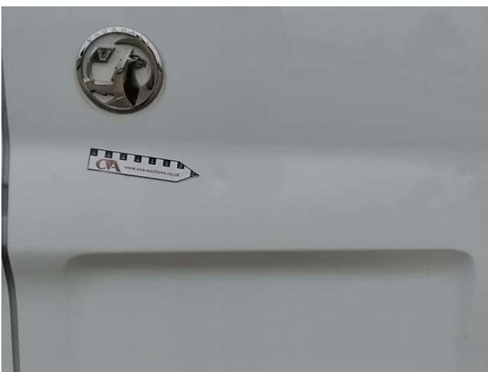
13: Door osr Dented Over 2 UpTo 10mm
