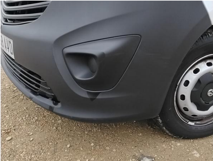
3: Bumper Front Moulding Scuffed (Unpainted) UpTo 100mm
