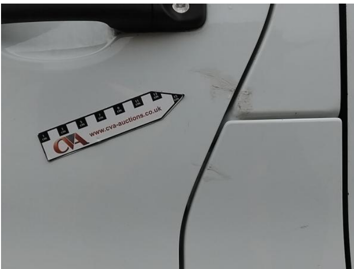
7: Door nsf Scratched Over 25mm Thru Paint
