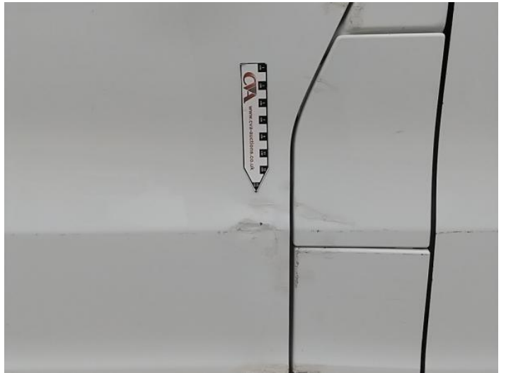
6: Door nsf Dented With Paint Damage
