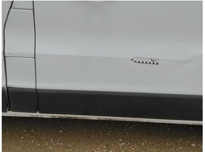
10: Door nsr Scratched Over 25mm Thru Paint
