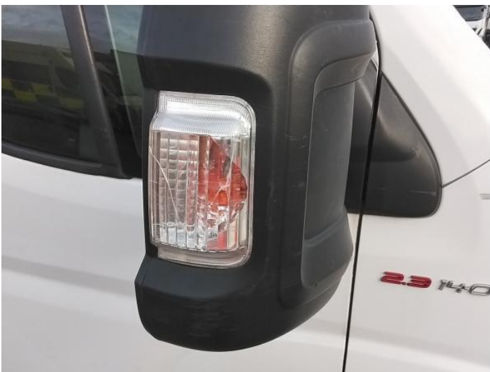
7: Door Mirror Assy osf Broken Replace
