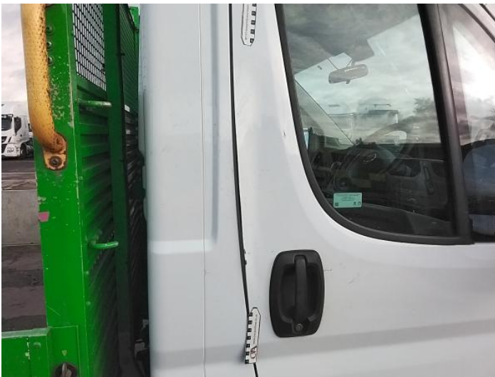
5: Door osf Dented With Paint Damage
