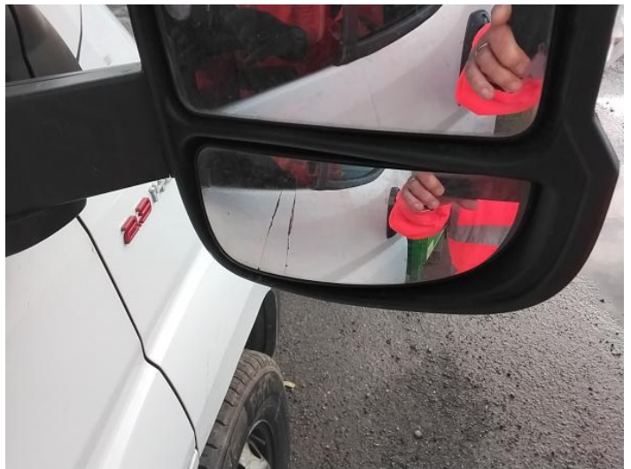
6: Door Mirror Glass os Broken Replace
