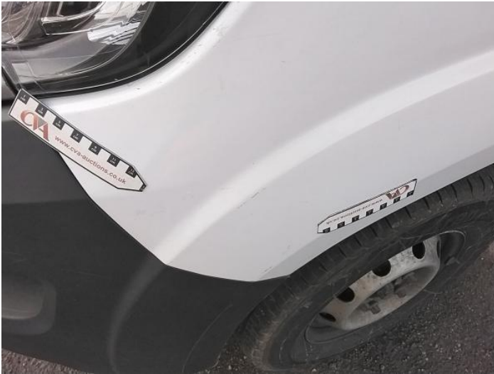
3: Wing nsf Scratched Over 25mm Thru Paint
