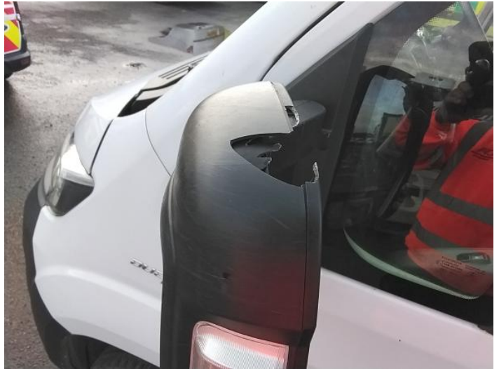
4: Door Mirror Assy nsf Broken Replace
