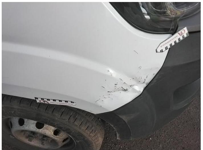
8: Wing osf Dented With Paint Damage
