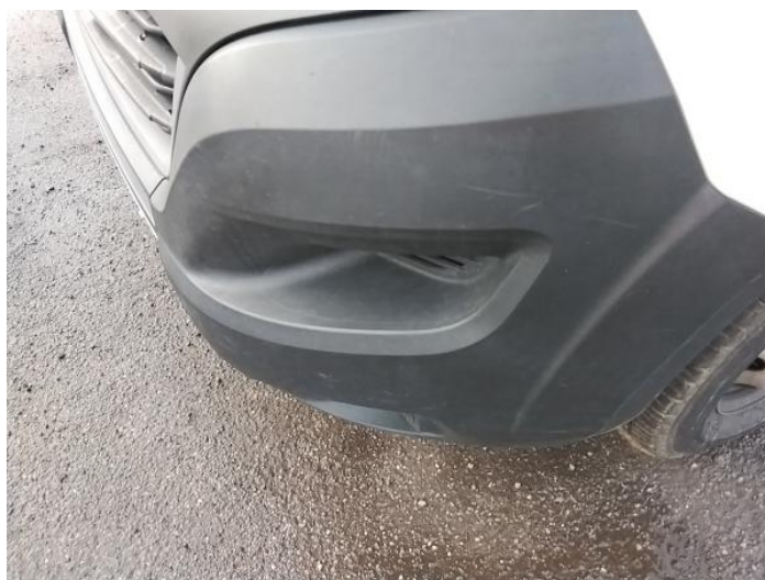
2: Bumper Front Moulding Scuffed (Unpainted) Over 100mm
