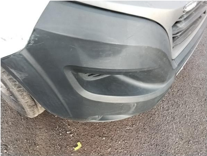
9: Bumper Front Moulding Scuffed (Unpainted) Over 100mm
