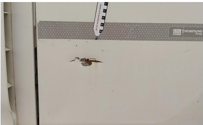
5: Bumper Front Dented Between 10mm + 30mm
