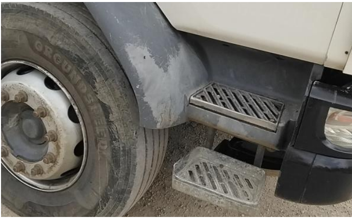
9: Wing Front Arch Extension ns Scuffed (Unpainted) Over 100mm
