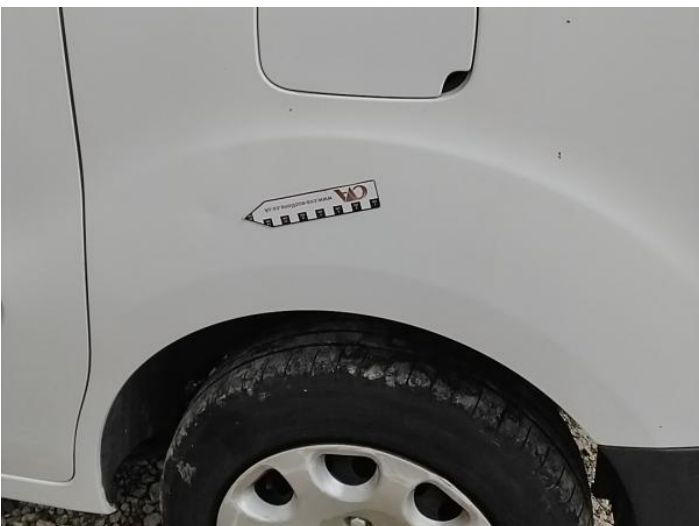
4: Qtr Panel nsr Dented Over 2 UpTo 10mm
